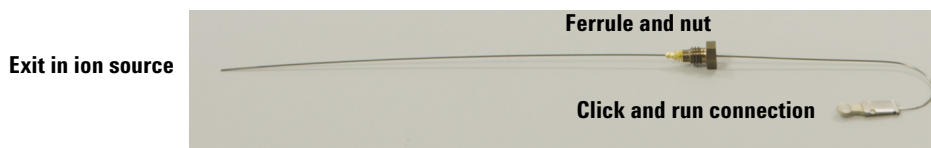
Figure 17 9000 GC/MS Tail removed from GC/MS Interface
