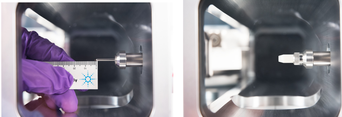
Figure 5 Installing a capillary column in the GC/MS interface for an EI EXT, SS, Inert, or CI source.
