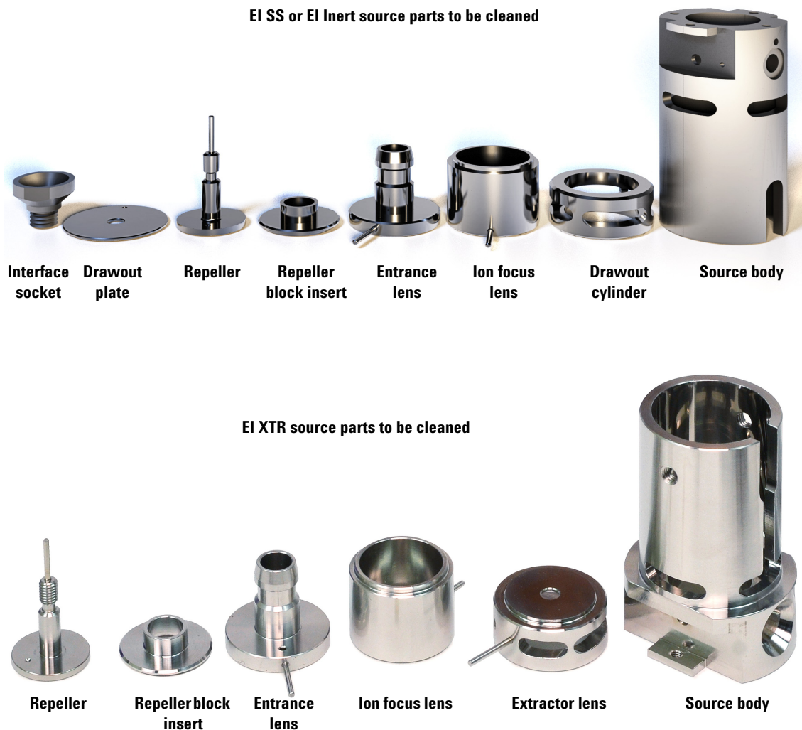
Figure 58 Source parts to be cleaned
