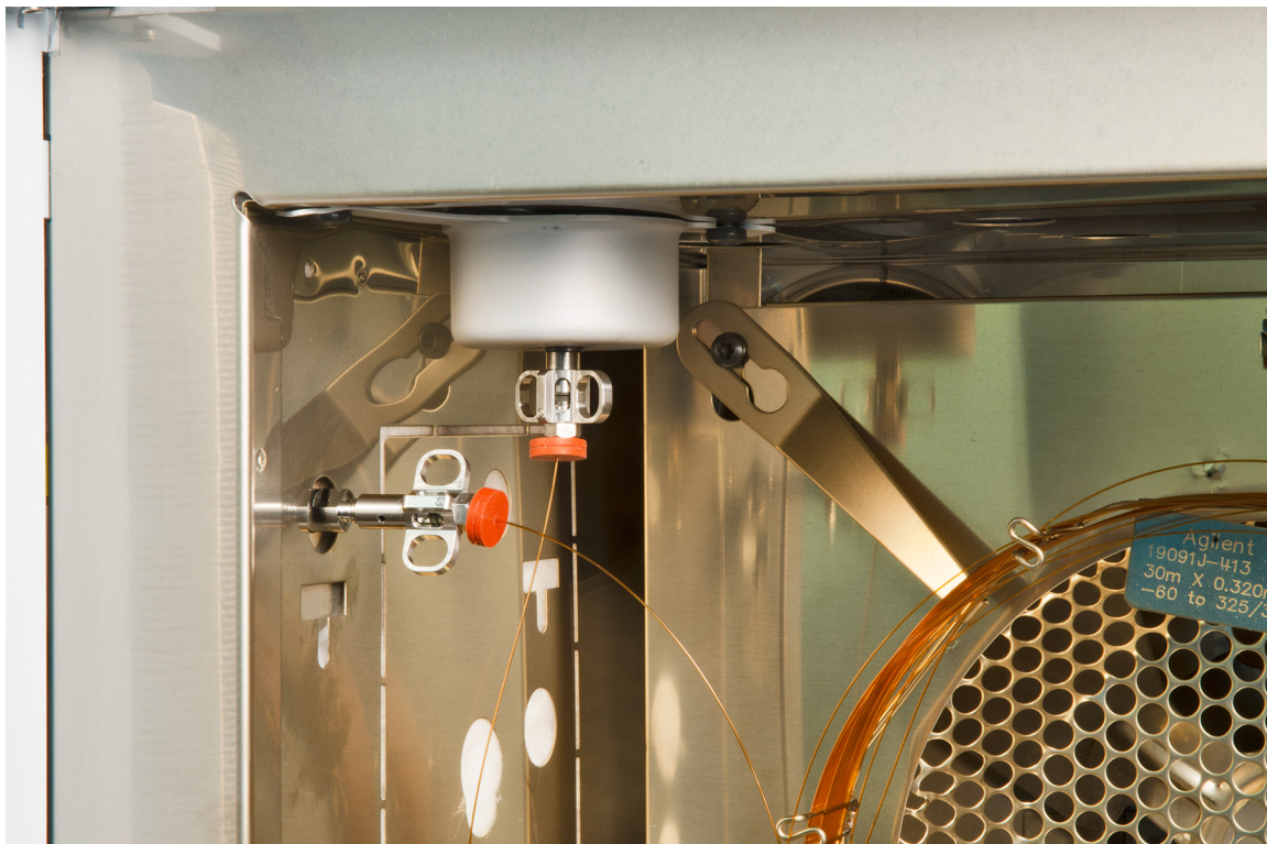
Figure 7 Installing a capillary column in the GC/MS interface
